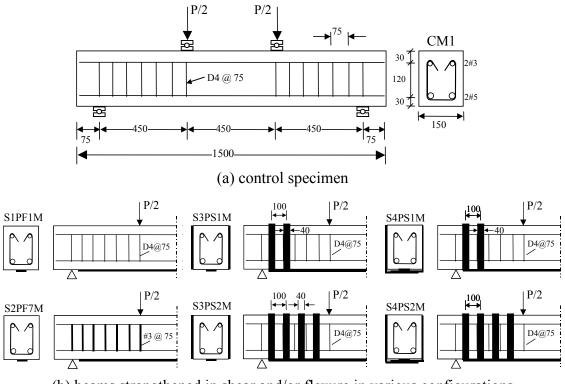
(b) beams strengthened in shear and/or flexure in various configurations
