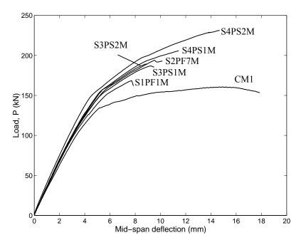
FIG. 3. Load-deflection curves of tested beams
