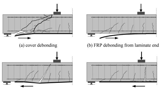
(c) FRP debonding from flexure-shear crack
