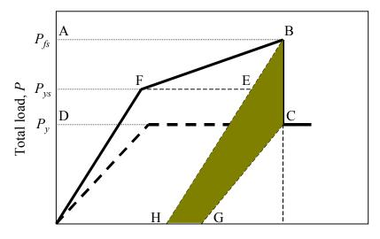
Beam deflection under load points,  $\delta_L$ FIG. 4. Potential energy difference in the beam upon debonding failure
